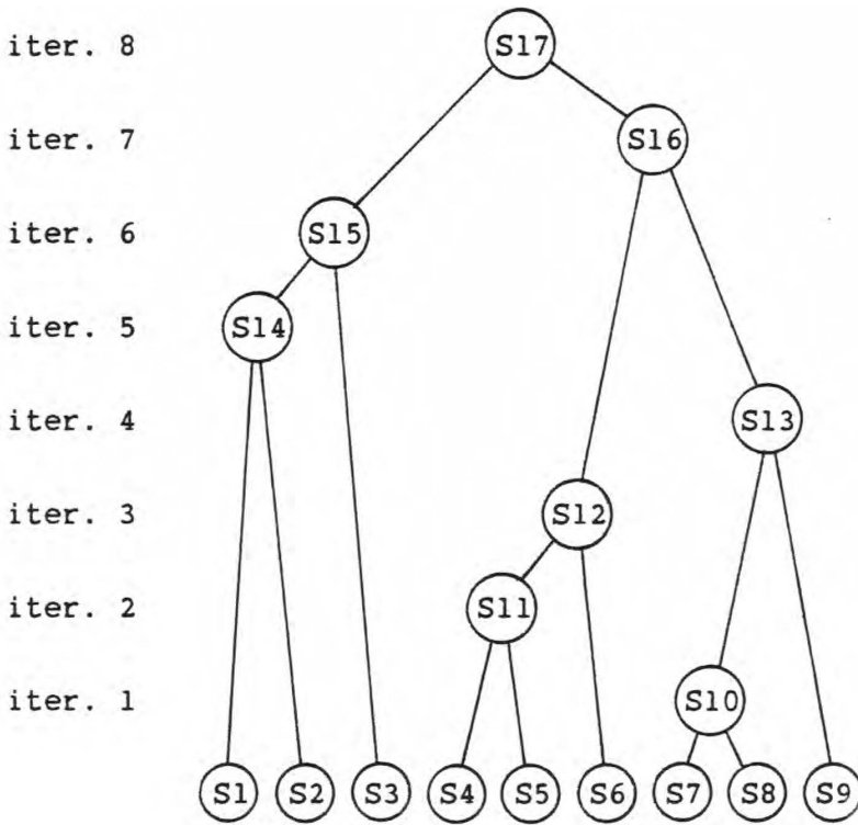
Figure 7.4: Sequence of segment merges for planar approximation.
